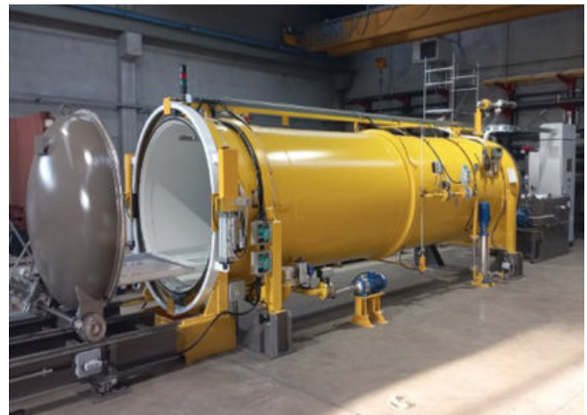
° Vaaro treatment pressure vessel.
